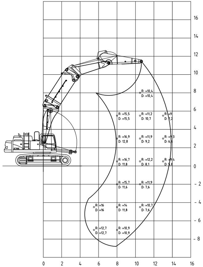
The above loads are according to the hydraulic excavator lift capacity ratings standard ISO/DIS 10567, they do not exceed 87% of hydraulic lifting capacity
