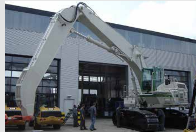
Example 2 – Material handling front, Hitachi EX1200
