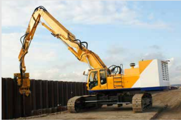
Example 2 – Telescopic sheet piling front, Etec 880
