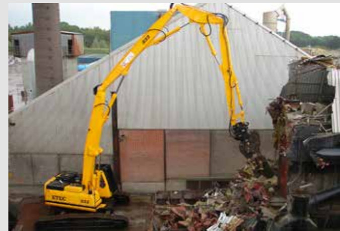
« Example 3 – Four piece high reach demolition front, ETEC 333
