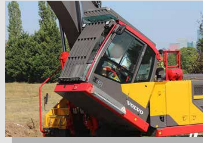
» Example 2 – Side Impact Protection (SIP), Volvo EC300
