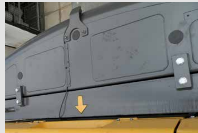
«« Example 3 – Sandwich mounted removable counterweight, Volvo EC700
