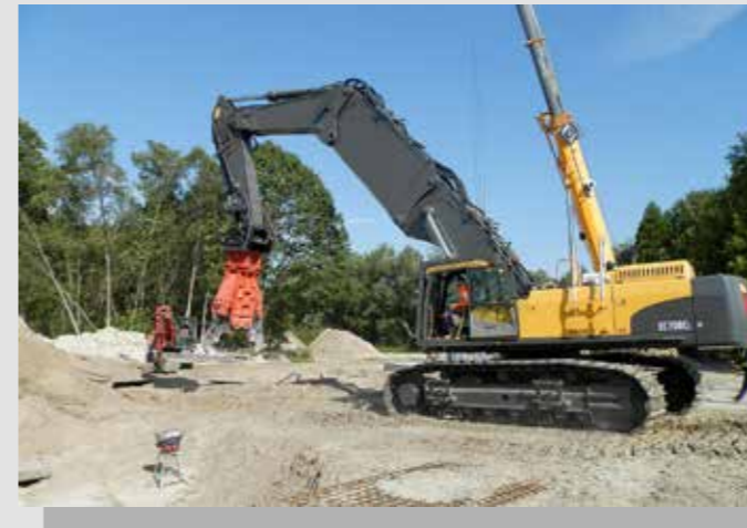
» Example 2 – Boom adapter Volvo EC700 with HRD front
