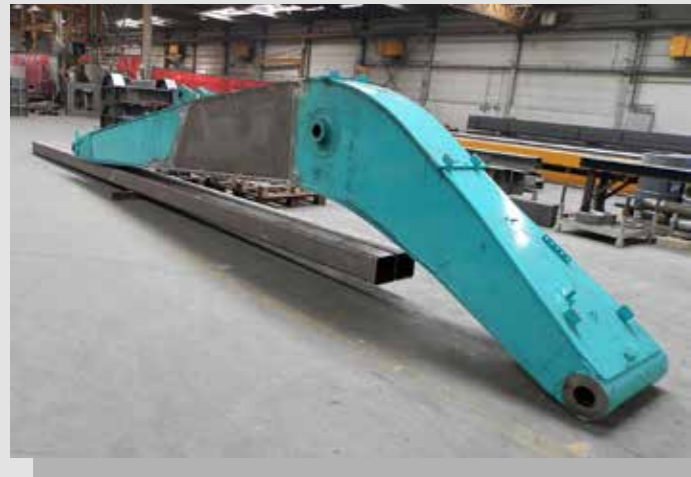
Example 2 - Extension of mono boom and arm, Hitachi ZX470 »»
