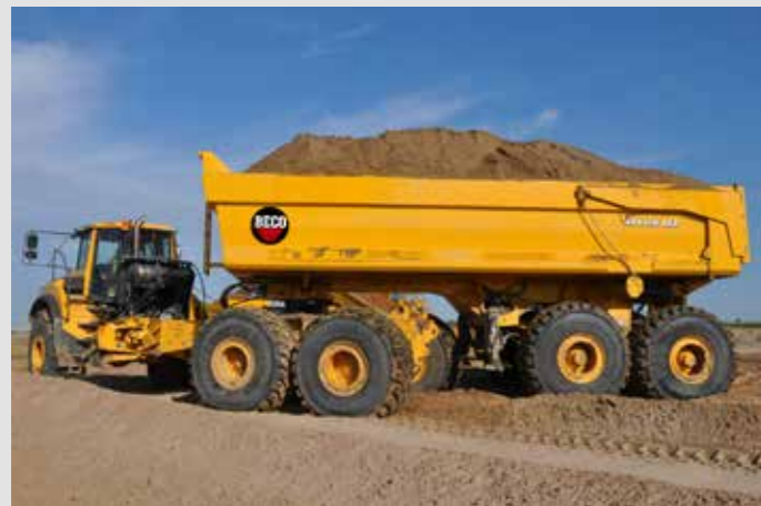
«« Example 3 – Semi dump trailer for 40 t articulated dump truck Volvo A40F
