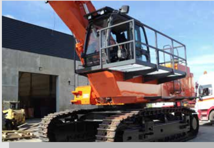
» Example 2 – Hydraulically elevating cab, Hyundai 360
