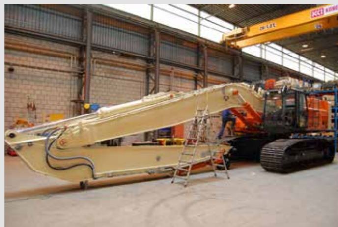
Example 2 - Extension of mono boom and arm, Hitachi ZX470 »»
