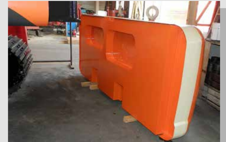
«« Example 3 – Sandwich mounted removable counterweight, Volvo EC700
